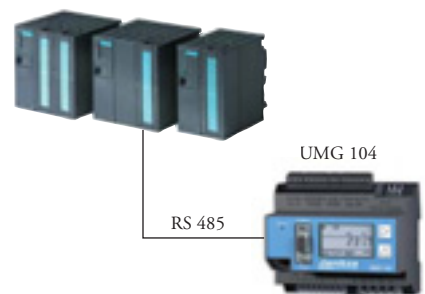
Example PLC communication with Profibus or Modbus
